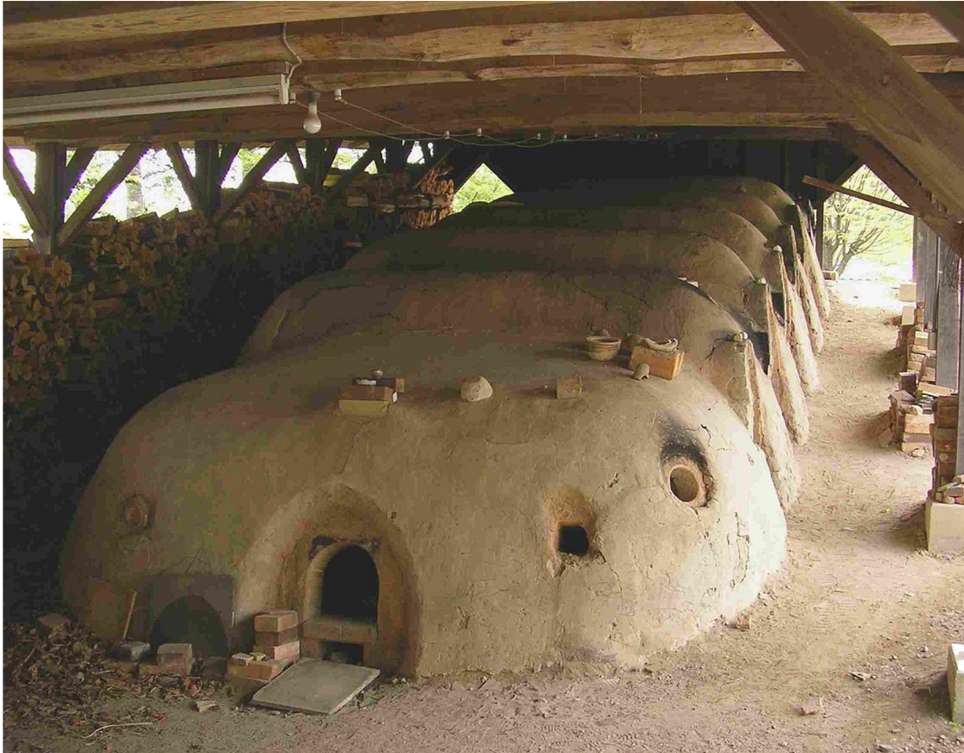
> japanese anagama kiln - also called dragon kiln collaborative firing for up to 12 days +3 weeks of cooling
